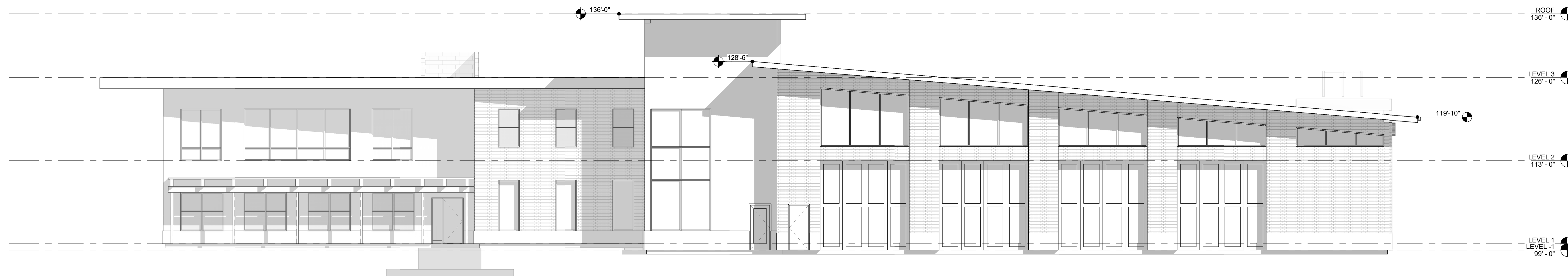
2 EAST ELEVATION - FIRE STATION 1/8" = 1'-0"
