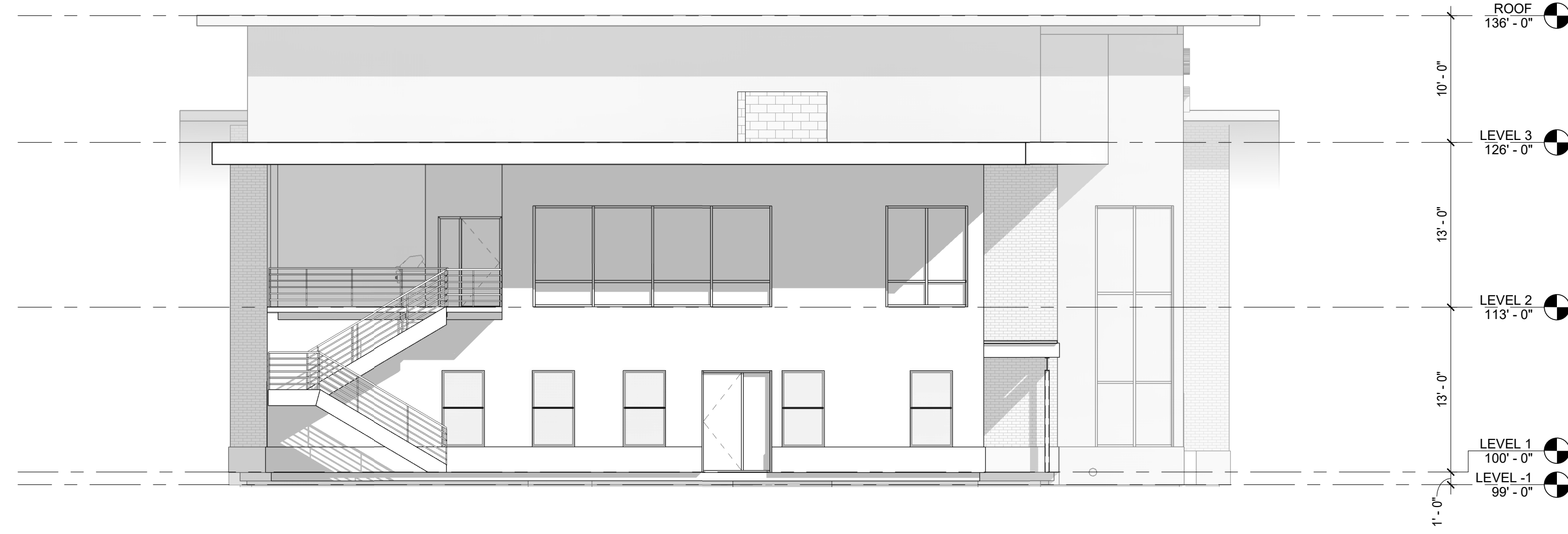
1 SOUTH ELEVATION - FIRE STATION 1/8" = 1'-0"
